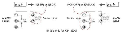
With the basic model of K34 (48x48), caution is required when using it alarm output. When control output is being used as a relay, the alarm output will be SSR output (voltage pulse). In this case, use SSR or alarm option (S10, S30) enabled models.
