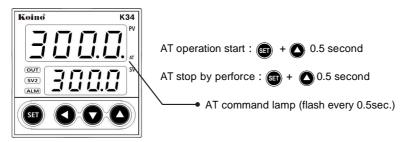
Tuning is required before operating for the first time. Set the target value(SV) in the range mainly used and run auto-tuning. When auto-tuning begins, the "auto-tuning command lamp" will flash every 0.5 second and will turn off upon completion of the tuning process. Please refrain from operating the keys while auto-tuning is in progress.
